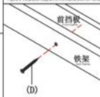
图4:扶手和铁架安装示意图 Figure 4: installation diagram of armrest and iron frame
